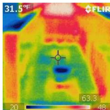
Next we take a look at a typical roof vent, where we see from the thermogram that it is venting so much warm indoor air when it is 33.3°F outside. It is actually taking the temperature of the base of the vent upwards to 63.3°F, almost to room temperature.
